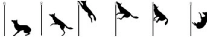
Figure 9. The Coyote Roller™ prevents coyotes from being able to get the foothold necessary to hoist them over a fence. (From Coyote Roller™)
